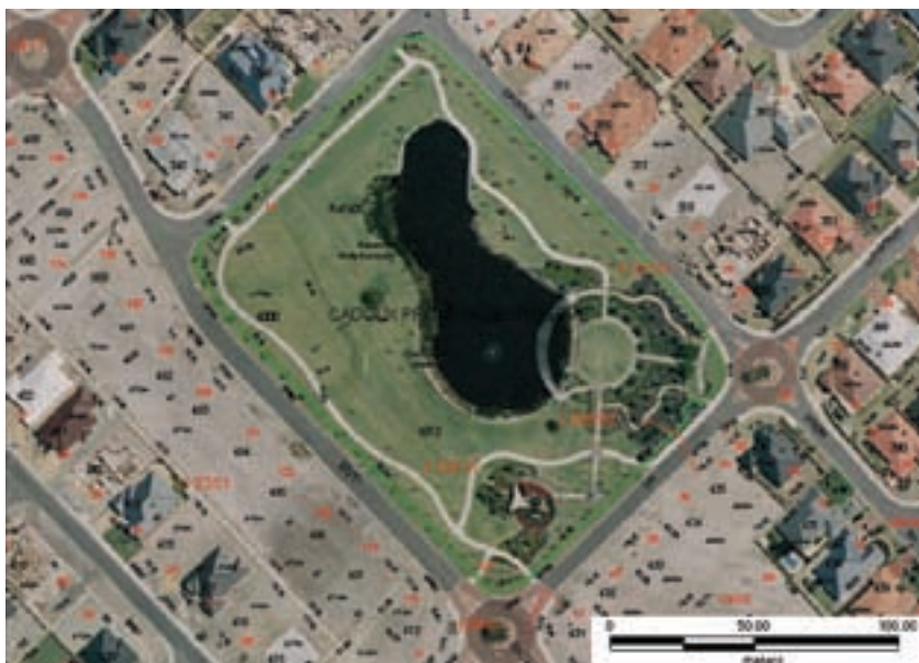
Photo 1: By locating the water body in the centre of the parkland, buffer distances to surrounding houses have been maximised. In addition space is available for planting screening vegetation between the water body and houses.
